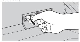
• Do not remove the SD Memory Card while the Access Indicator is flashing.
